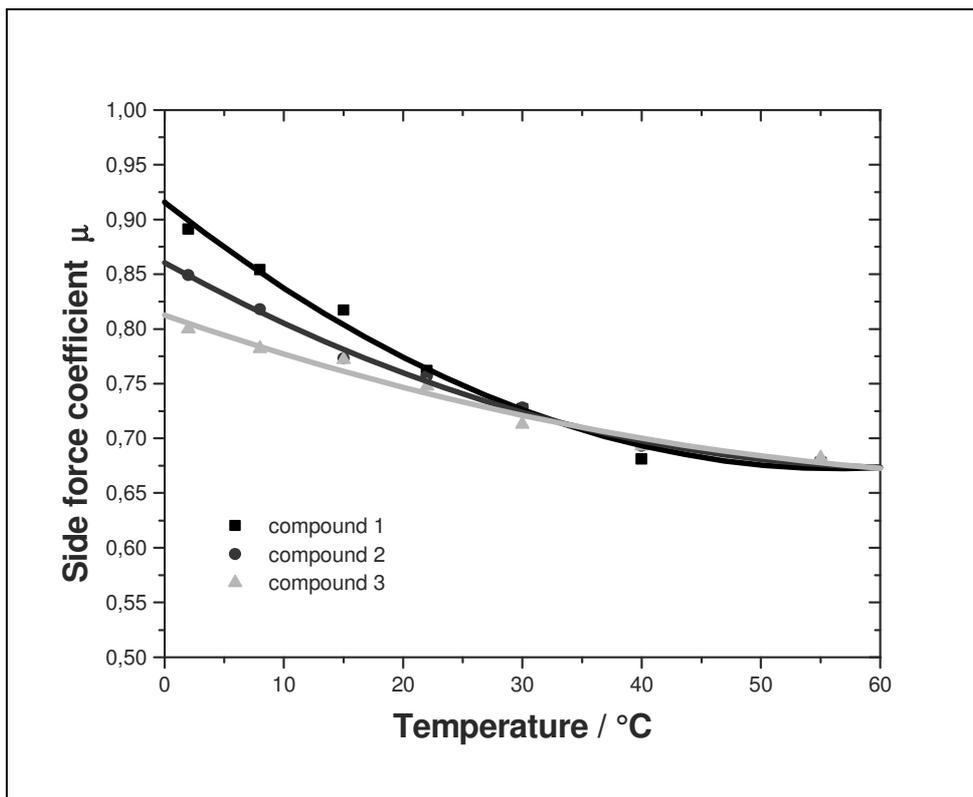
Figure 6 – Side forces dependency on temperature
