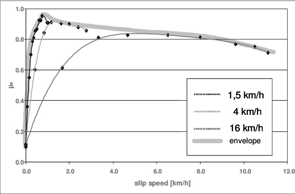
Figure 8 – Envelope of  $\mu_s$  for different test parameter sets for a silica compound
