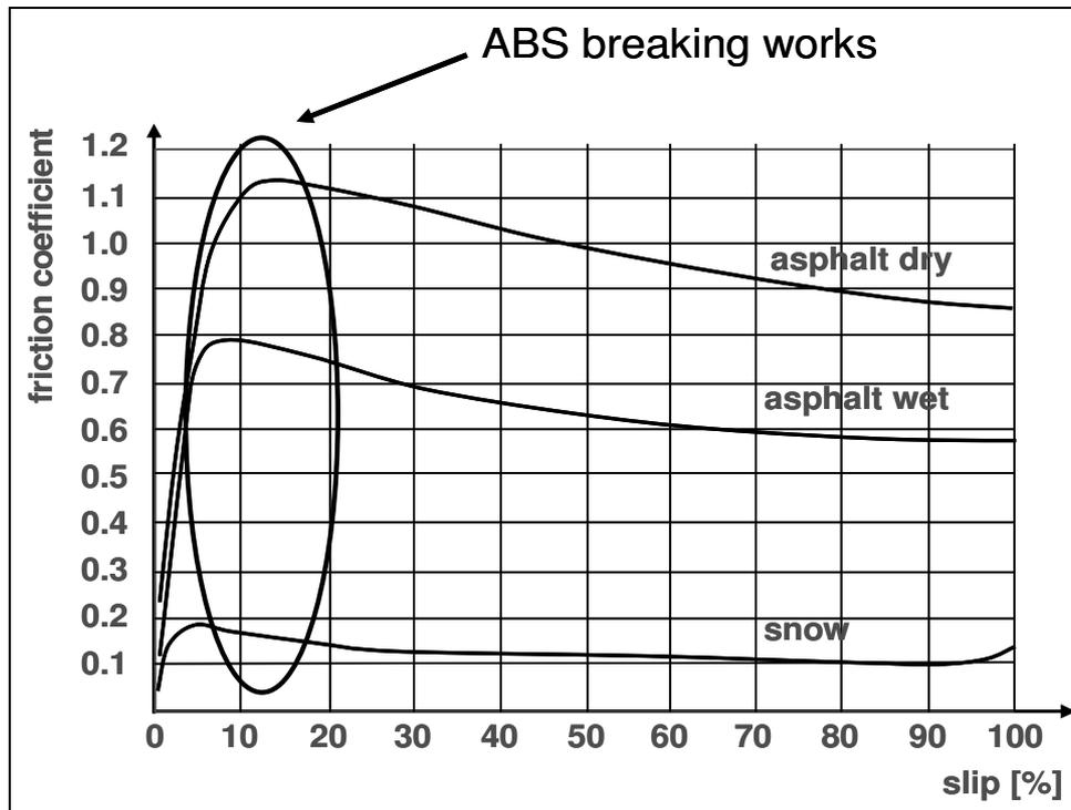
Figure 1 – Friction coefficient for different road surface conditions
