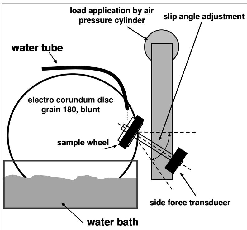
Figure 4 - Arrangement of the test equipment
