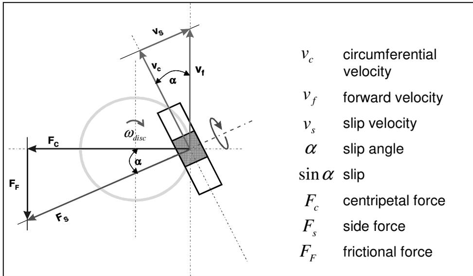
Figure 5 – Velocities of the sample wheel and the resultant forces
