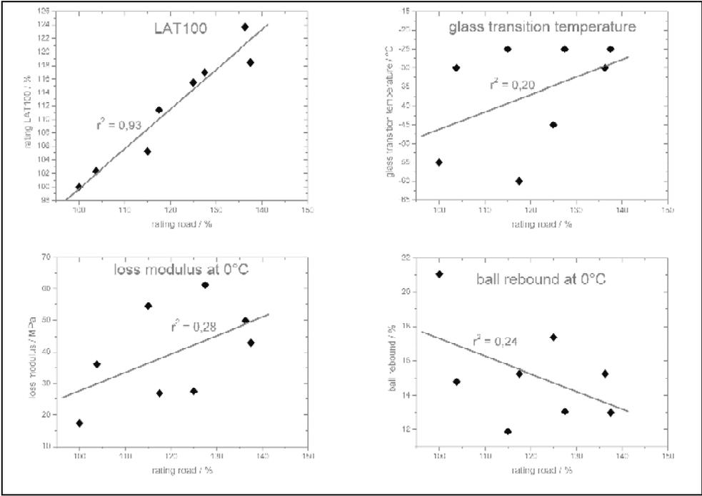
Figure 11 – Comparison between tire tests, LAT 100 and other rubber tests for winter tire tread compounds
