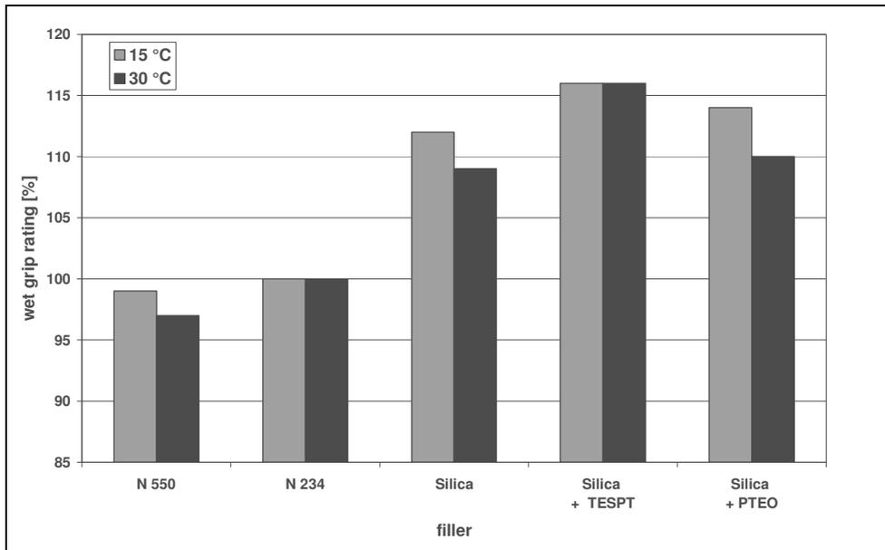
Figure 10 – Wet traction results of carbon black and silica in an S-SBR compound
