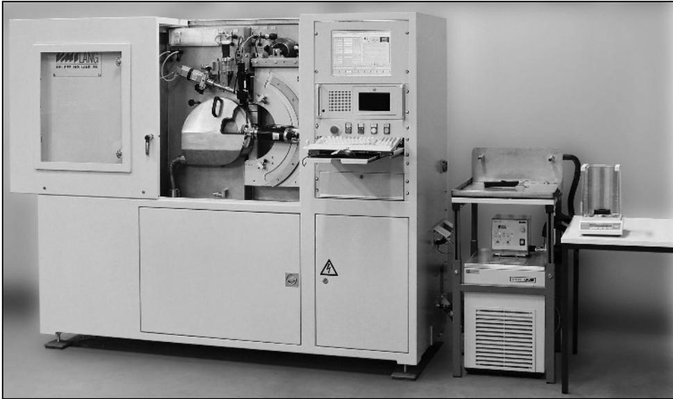
Figure 3 – Photograph of the test equipment (LAT 100)
