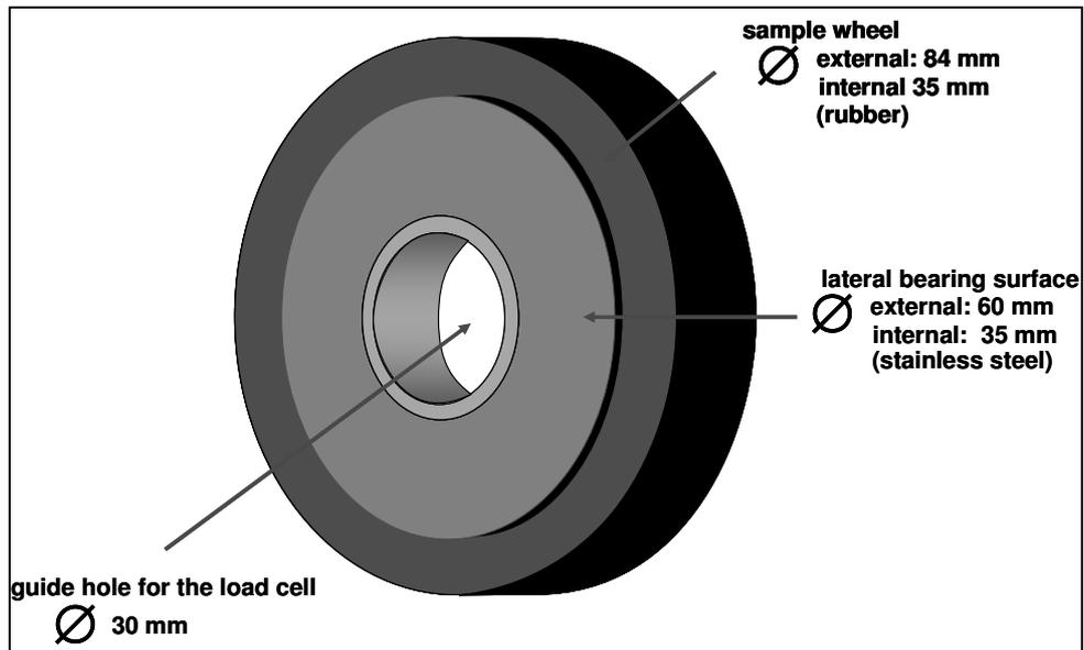
Figure 2 – Test specimen including bearing facilities
