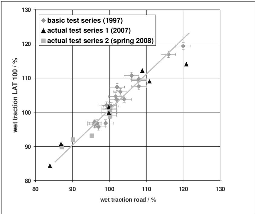
Figure 12 – Comparison between tire tests and LAT 100 results for summer tire tread compounds
